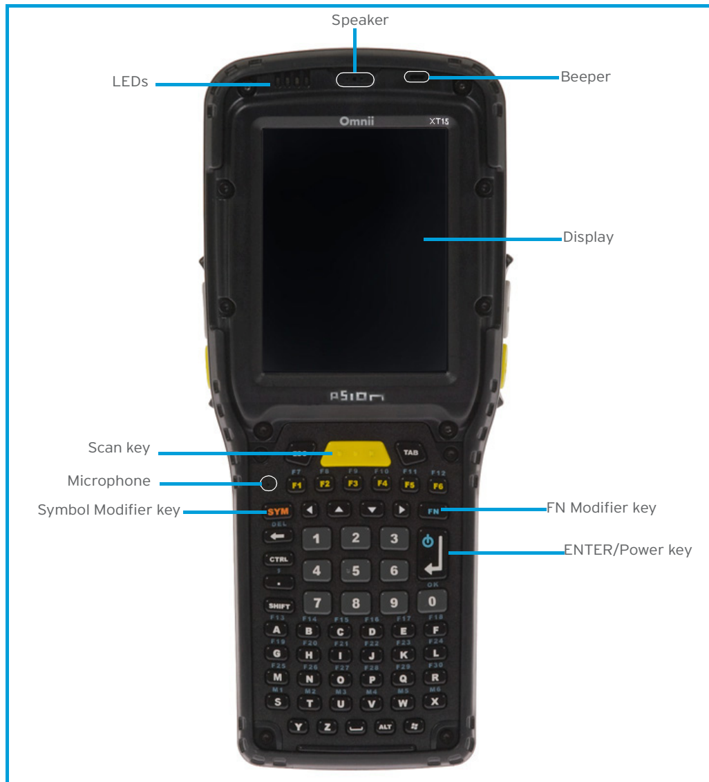
Figure 2.1 Front View of the Omni XT15 Model with Alphanumeric Keyboard
