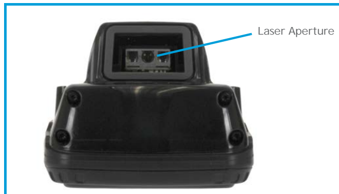
Figure 1.3 Top View (Scanner Window)
