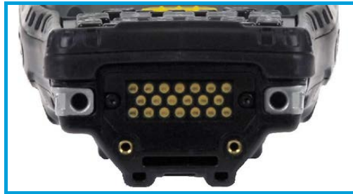
Figure 1.2 Bottom View (Docking Connector)
