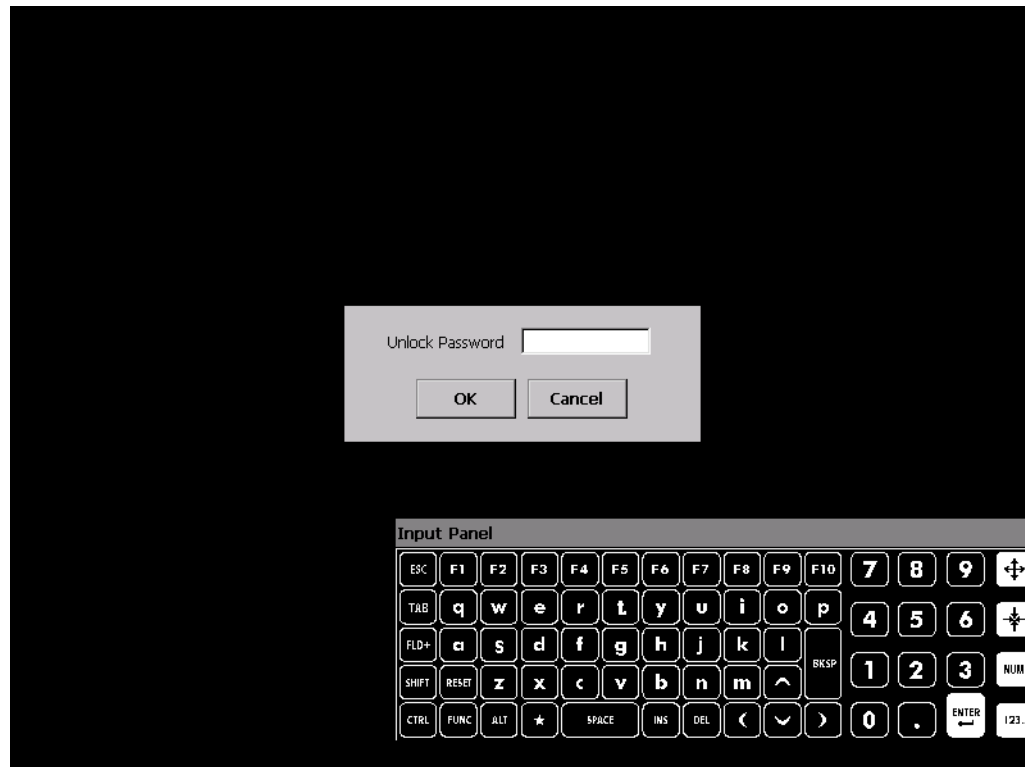
Figure 2-54 Terminal Lock Over-Ride
